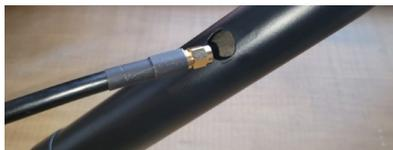
Once threaded, pull the cable through the pole leaving enough at the top end of the pole to connect the antenna via the screw on SMA connector. Once the remaining cable is fed through the pole add the second grommet to the rear of the bracket. Now connect the antenna using the screw type SMA connector and feed any excess cable back down the pole.
