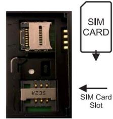
The larger slot is the SIM card slot please insert the SIM face down with the cut off corner in the same position as on the marking in the SIM tray. Once the SIM has been inserted under the retaining bar, insert the battery and fix the back plate to the router.
