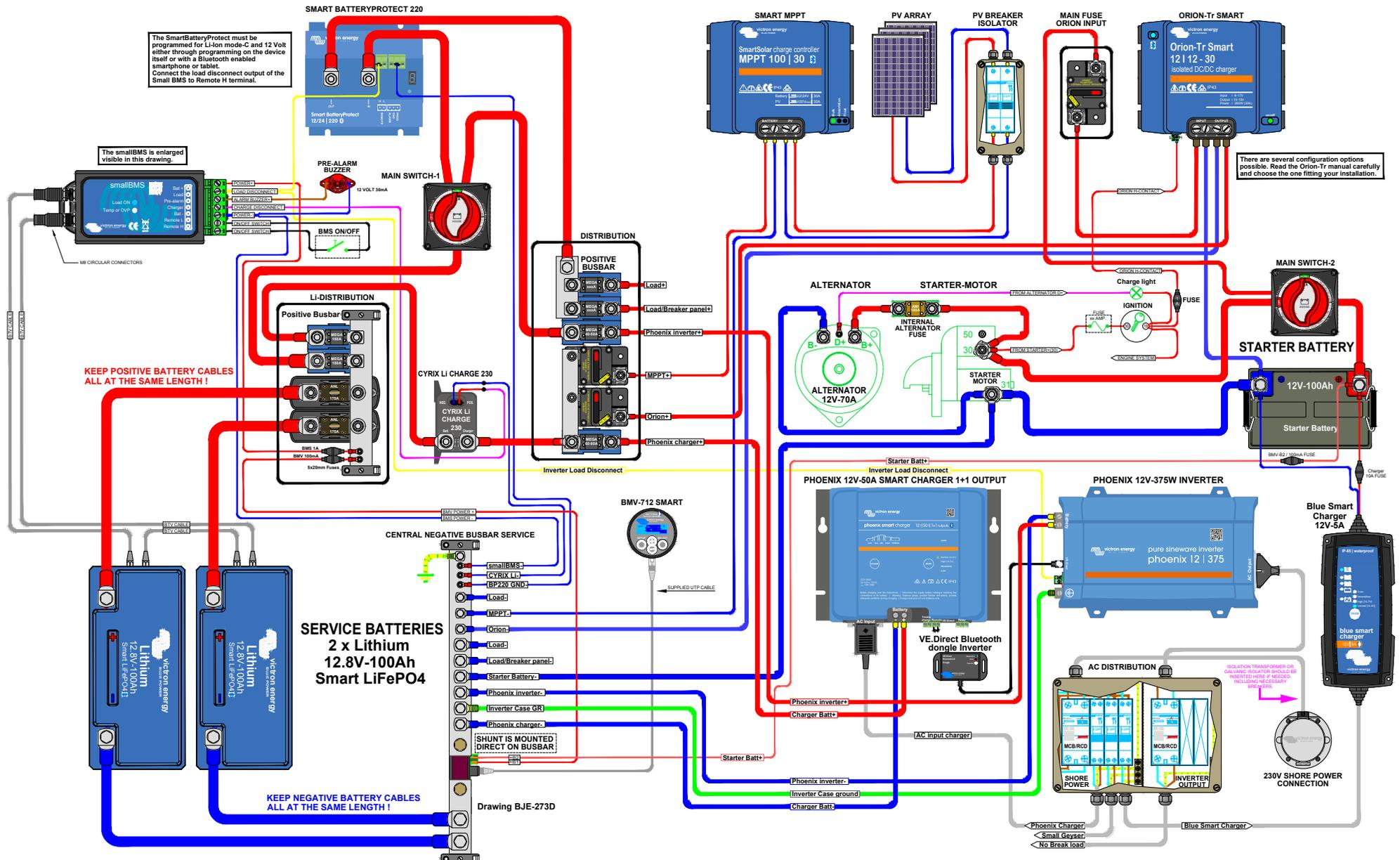
The SmartBattery/protect must be programmed for Li-Ion mode-C and 12 Volt either through programming on the device itself or with a Bluetooth enabled smartphone or tablet. Connect the load disconnect output of the Small BMS to Remote H terminal.
